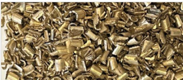
Fig. 5: Rg7 (CC493K) chip with industrial machining
