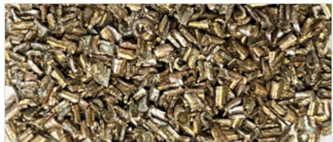
Fig. 6: EC7 chip with industrial machining
