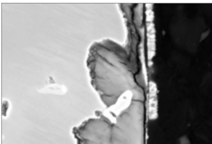
Fig. 7: Corrosion behaviour of Gbz12 (CC483K) in salt water at room temperature over 168 hours
