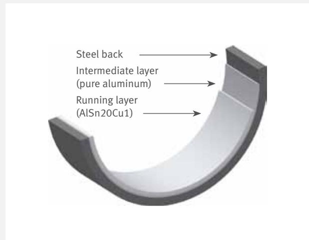
Bi-material: steel / aluminum bearings
