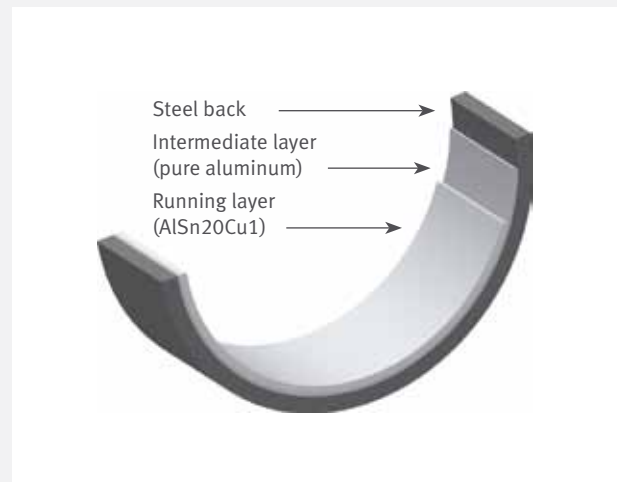
Bi-material: steel / aluminum bearings
